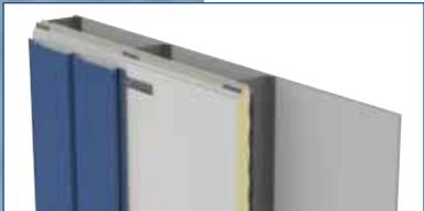
**HPCI Barrier™ Wall Panel** – The HPCI Barrier metal wall panel is an air, water, thermal and vapor barrier panel that can be used behind any type of façade. Installed in a horizontal orientation, completely outside of structural supports, there are no thermal bridges to reduce energy efficiency. The interior profile is Mesa. R-values of up to R-28.6 can be achieved with the HPCI Barrier Wall Panel.
