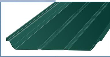
**Ultra-Dek® Roof Panel** – Ultra-Dek is a 24" wide snap-together, trapezoidal leg standing seam roof system. It is ideal for industrial, commercial and architectural applications. The standard offering for the Ultra-Dek system is a sliding clip that allows for thermal movement. Ultra-Dek panels can be installed on various types of construction. Recommended for roof slopes of ¼:12 or greater.
