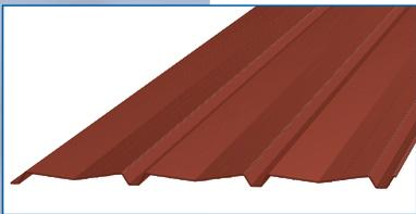
**AVP Wall Panel** – AVP is a 36" wide panel with semi-concealed fasteners. The panel profile produces a decorative shadow line resulting in a distinctive architectural effect. Ribs are 1 ⅞" deep and major corrugations are spaced 12" on center. The attachment of the panel is made from the exterior with color matched fasteners. Available in 26 and 24 gauge.
