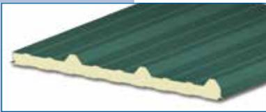
**LS-36™ Roof & Wall Panel** – The versatility of the LS-36 insulated metal roof and wall panel offers a multitude of design options. The overlapping, through fastened joint allows for quick installation. The exterior profile features 1 ¼" high major ribs at 12" centers with Mesa in between ribs at 4" centers. The interior skin has a Mesa profile. LS-36 offers R-values to R-42.9.
