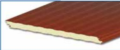
**Mesa Wall Panel** – The Mesa panel is well suited for exterior wall and interior partition wall applications. The lightly corrugated Mesa profile on both faces of the panel ensures symmetry and uniform appearance from outside to inside and from room to room in partition applications. Mesa offers R-values of up to R-42.9.
