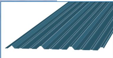
**PBR Roof and Wall Panels** – PBR is a 36" wide panel that works well for roof and wall, as well as liner, mansard and soffit panel applications. Its 1 ¼" deep ribs create an even-shadowed appearance and the area between the ribs is reinforced with minor ribs. The attachment of the panel is made from the exterior with color matched fasteners. Available in 26 and 24 gauge.
